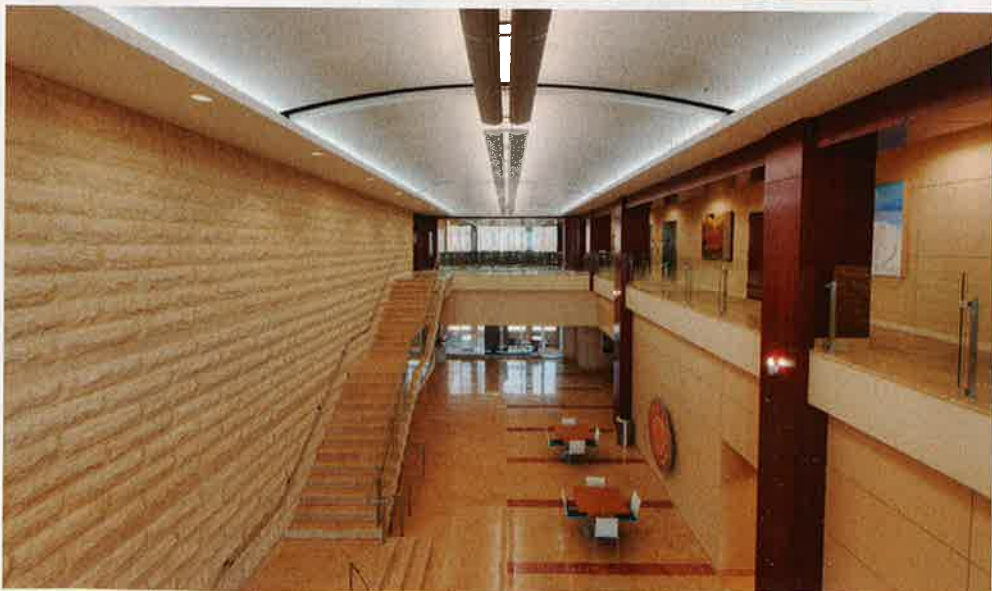
For the flooring and monumental stair in the atrium of the office building, a combination of Sunny Light and Khatameya (Sahara Beige) marble — both from Egypt — and Rojo Alicante marble from Spain were employed.
